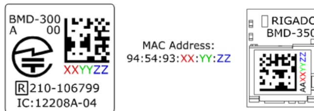
Figure 3. Where to Find MAC Address on BMD-300 Series
